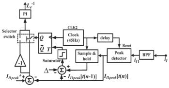
Fig 3.5: Schematic block diagram of the feedback loop which sets the value of the emulated inductance.
