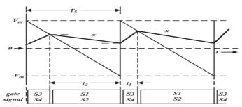
Fig 3.2:Carrier waveform (sawtooth), modulating waveform x, and gating signal
