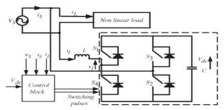
Fig 3.1: Schematic Block diagram of single phase Active Harmonic filter systems
