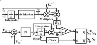
Fig 3.4: Block diagram of the controller for existing system
